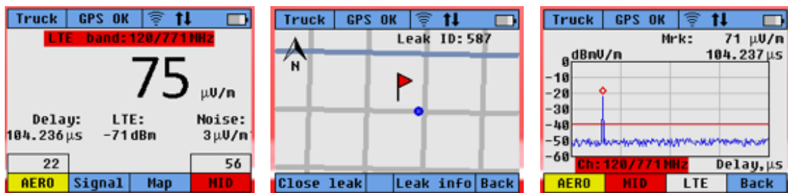
FIGURE 2 CORRELATOR RESPONSE, DETECTED VIEW AND MAP VIEW
