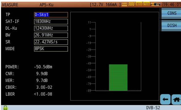
Figure 9: DVB-S/S2 Signal Measurement
