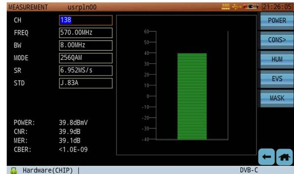
Figure 12: DVB-C Signal Quality Measurement
