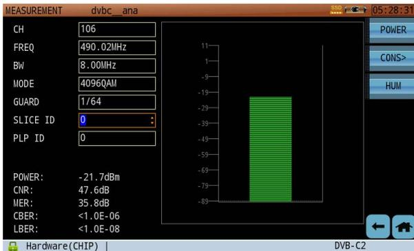
Figure 16: DVB-C2 Signal Quality Measurement
