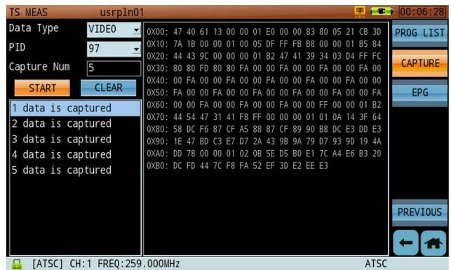
Figure 40: PID Capture
