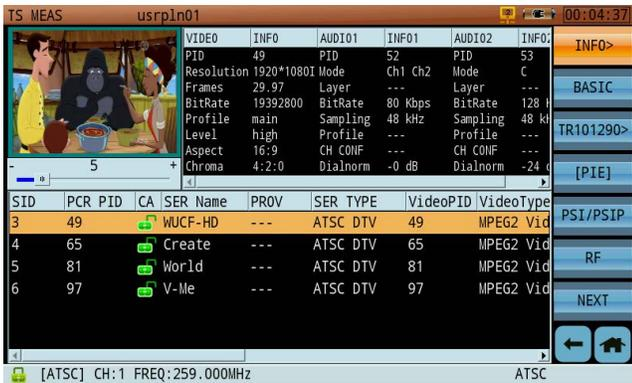
Figure 30: Programs Decode Monitoring & List
