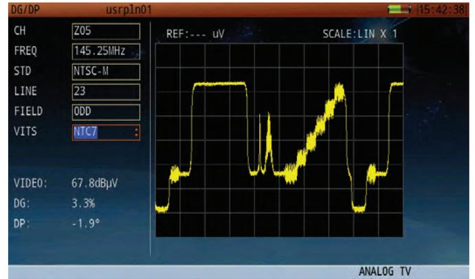
Figure 8: Analog TV Gated Measurement: Video Parameters
