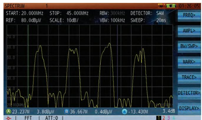
Figure 4: Spectrum Analysis - Low-Level Signal Covered by High-Level
