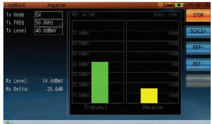
Figure 22: Loopback Measurement
