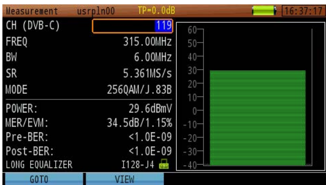
Figure 3: DVB-C Channel Measurement
