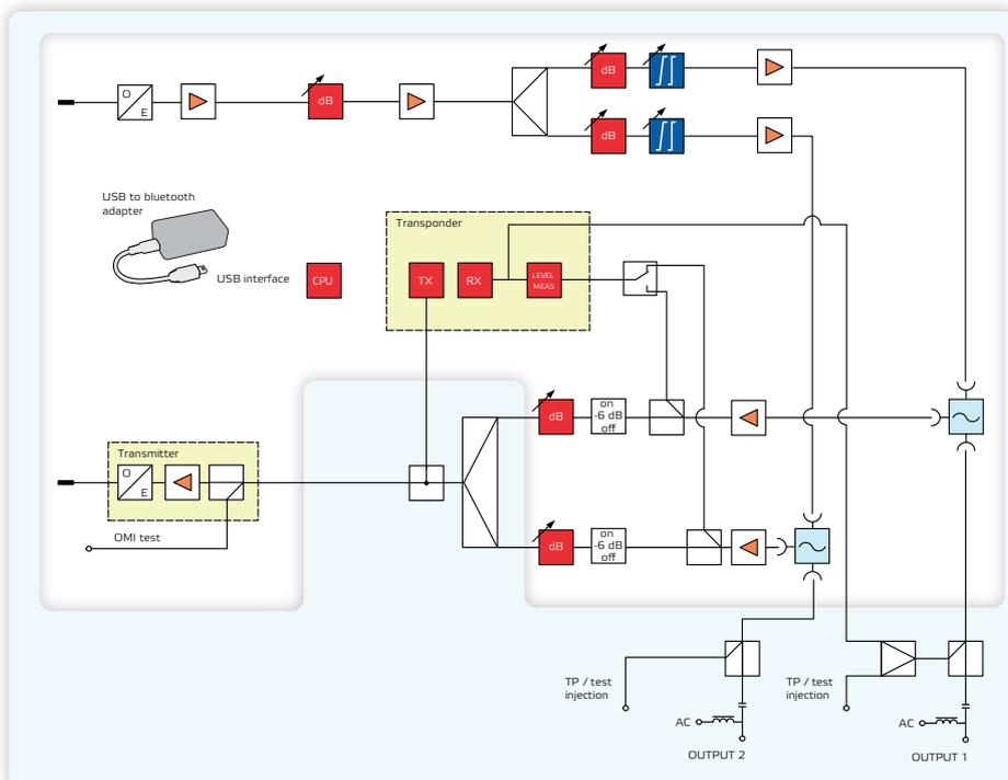
The output amplifier stages use high performance GaN hybrids, which makes the usable output level range especially wide.
