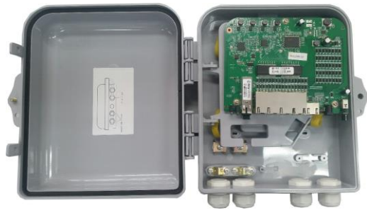
CGR8ONU INTERNAL VIEW
